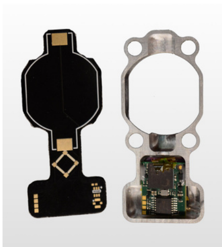
Gages installed directly on aluminum circuit board in a fully integrated torque monitoring telemetry module
